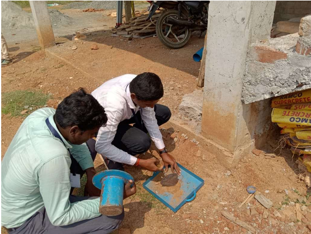
FIELD DENSITY TEST OF SOIL BY SAND REPLACEMENT METHOD FOR SOIL COMPACTION
